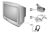
Depending on the versions, the connectors are located on the front (sometimes under a flap) or on the right-hand side of the TV set. Make the connections as shown opposite. With the key, select AV.
